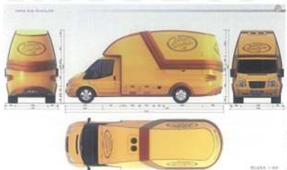
Corba satıs Aracı, inox, fiberglass, metal profil, 6720x 2145x 3120 U x G x Y Mobile Soup Truck, inox, fiberglass, metal profile, 6720x 2145x 3120 U x G x Y
